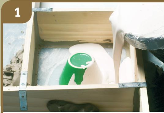
**1** Ensure the object to be cast does not have any undercuts as this method of mould making will create a single pull mould. Place the object to be moulded on a non-porous surface. Seal all the gaps of the mould making frame with spent clay. Ballast the frame walls with extra blocks of clay. Mix the plaster (835g plaster to 1 pint of water) and pour over the object to be cast. Leave the plaster to set.
