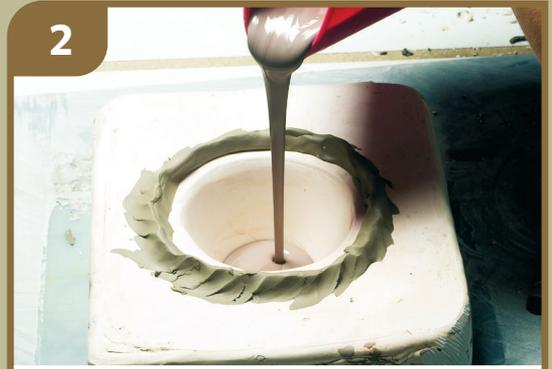
**2** Once the plaster is dry, remove frame and object from the mould. Moulds should be left until bone dry. For slip casting, build clay edge up around the rim of the mould. Mix casting slip thoroughly then tip into the plaster mould to just above the mould top. This allows for the excess to be trimmed away neatly.
