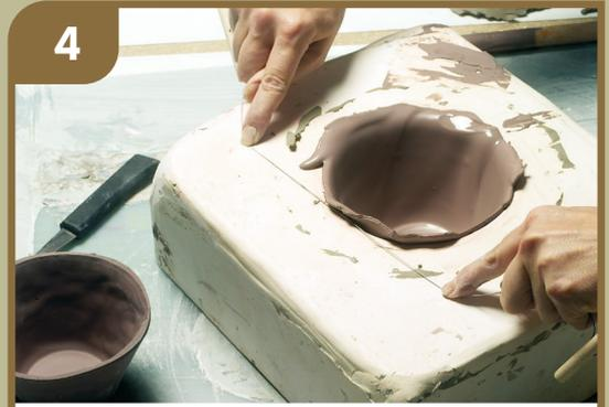
**4** Once you have the required thickness, pour out the excess slip into a reserve bucket. Leave the slip cast shape in the mould until it has begun to shrink and release itself from the plaster walls. Trimming around the top rim can be done with a clay cutter at the leather-hard stage. The piece can then be removed from the mould and coated with decorating slip or glazes.
