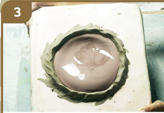
**3** The length of time the slip is left in the mould depends on how thick the wall of the cast needs to be. A visual indication can be seen by looking at the change in colour of the slip around the edges of the mould or by moving the mould slightly to reveal the rim.
